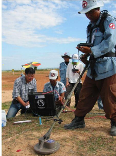
Fig.1. ALIS system in operation in CMAC test site, Cambodia in 2006. This is a VNA based ALIS, which is to be operated by two deminers. The sensor operator is observing a palmtop PC and the other PC operator is operating a Note PC. ALIS does not require the second operator, but the second operator can observe the operation of the deminer scanning the sensor, and also can advise for the detention by monitoring the visualized image of GPR and a metal detector.
