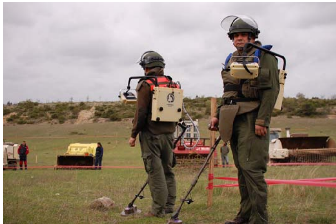
Fig.3. Pulse GPR based ALIS (ALIS-PG) .The system is almost the same as the VNA type ALIS. ALIS-PG is light weight, and scanning for GPR data acquisition can be faster than VNA type.
