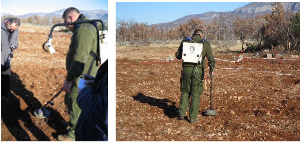
Fig.10. Hirvoje Stipetic and Nikola Gambiroza (CROMAC technical manager) QC after machine demining. The soil is plowed and many small rocks appear on the surface.
