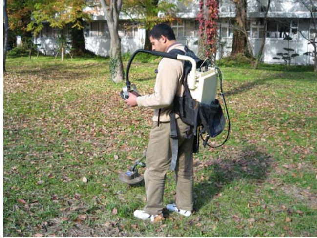
Fig.2. VNA based ALIS for a single operator. This ALIS can be operated by a single deminer. The deminer can observe the sensor scanned trace on the palmtop PC display in real time, and then the signal processing for 3-dimensional display of GPR data is achieved on the same PC. The deminer will interpret the GPR images to identify the buried mines.
