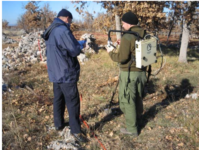
Fig.6 Interpretation of ALIS data. The deminer is observing GPR horizontal slice images on the palmtop PC display, after processing the acquired data sets. The signal processing for 3-dimentional GPR imaging takes about 10second.
